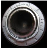
**On left-hand side in direction of travel: Left-hand thread**
